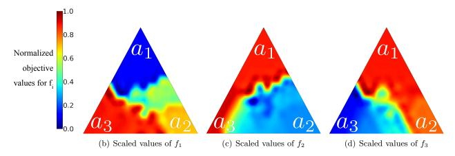
FIGURE 5 A grid exploration over the ternary graph. An optimization was conducted for a grid of coefficients regularly spaced on the ternary graph. The resulting scalarized objective is decomposed into the constituent objectives (normalized between 0 an 1) and plotted on separate summary ternary graphs.
