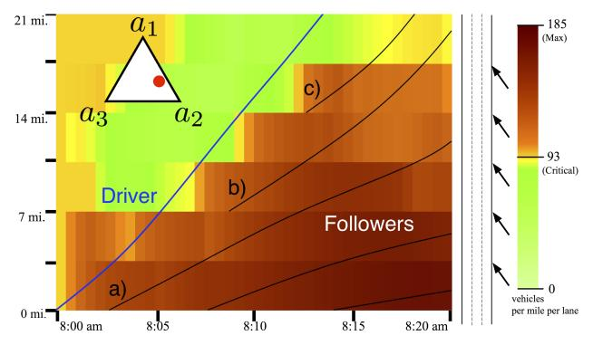
FIGURE 4 Space-time diagram with a ternary graph representing the  $a_1, a_2, a_3$  coefficients (here 30%, 55% and 15% respectively) used for the scalarization process in the catch-me-if-you-can example. The trajectory of the driver (blue line) appears to always gain distance in relation to pursuants further upstream (black lines). Best viewed in color.
