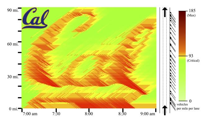
FIGURE 3 Space-time diagram obtained following a *congestion-on-demand* attack with a Cal logo as the objective. The attack was simulated on a 90 miles and 33-onramp freeway, for a 2 hours simulation time and using coordinated ramp metering.
