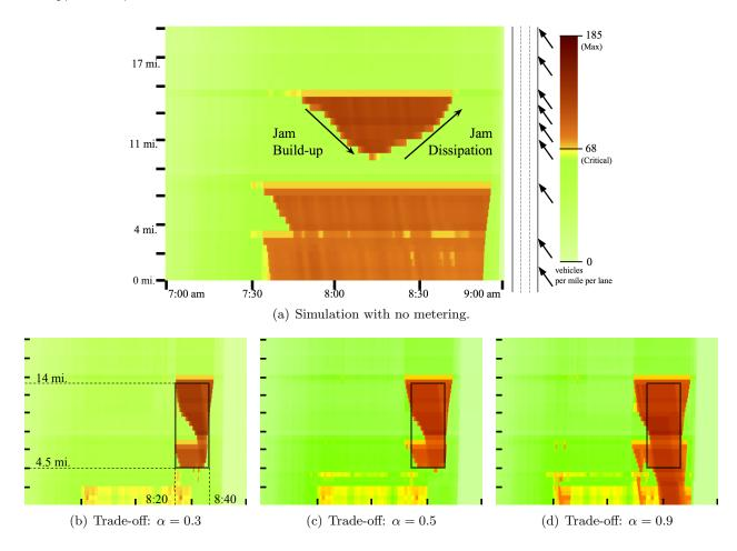
FIGURE 2 Figure 2(a) depicts a space-time diagram of vehicle densities on 19.4 mile stretch of I15 Freeway with no ramp metering. The box objective, and example of *congestion-on-demand*, is applied in Figures 2(b)-2(d). The user specifies a "desired" traffic jam between postmile 4.5 and 14, for a duration of 20 minutes between 8:20 and 8:40. For this, the  $\alpha$  parameter enables the proper design of tradeoffs in the objective.
