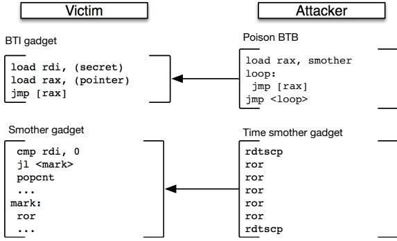
Figure 3: Overview of the SMoTHERSPECTRE components.
