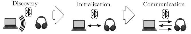
Figure 3: CTKD life cycle has three phases: Discovery (to exchange features), Initialization (to agree on a pairing key and, through CTKD, create a pairing key for the other transport), and Communication (to establish secure sessions on BT and/or BLE).
